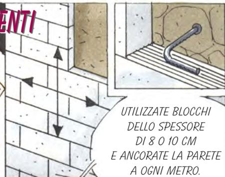
UTILIZZATE BLOCCHI DELLO SPESSORE DI 8 O 10 CM E ANCORATE LA PARETE A OGNI METRO.
