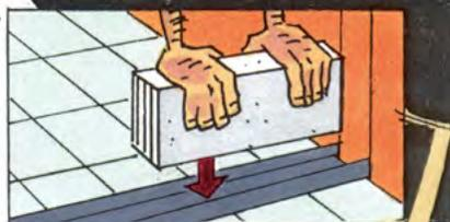
STENDETE LA MALTA COLLANTE SULLA SUPERFICIE INFERIORE E SU QUELLA VERTICALE DEI BLOCCHI PRIMA DI INFILARLI NEL PROFILO A "U".
